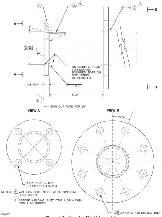
Figure 1-5. Abrasive Shield Assembly
